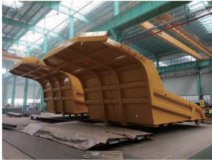
Finished mining truck compartments of XCMG
